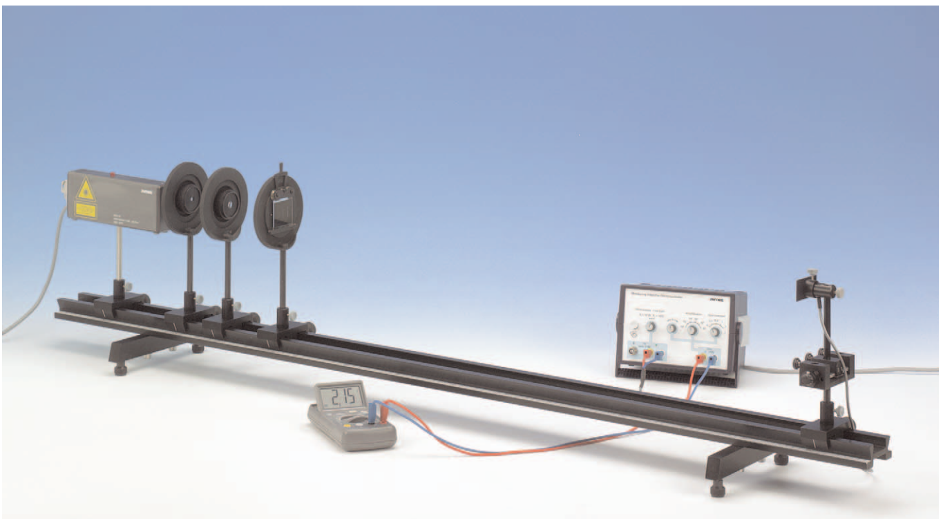
Fig. 1: Experimental set-up to investigate the diffraction intensity of multiple slits and grids. (Positions of the components on the optical bench: laser = 2.5 cm; f/20 mm lens = 14.5 cm; f/100 mm lens = 27.5 mm; diffracting objects = 33 cm; slide mount lateral adjustm., calibr. = 147.5 cm).
