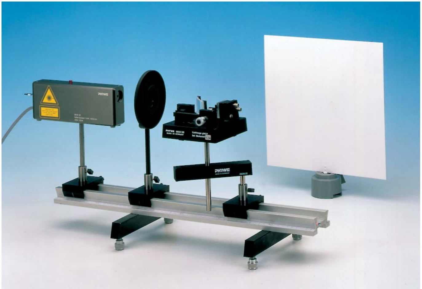
Fig. 1: Experimental set-up for measuring wavelengths with the Michelson interferometer.
